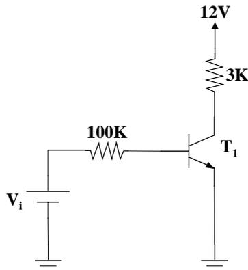
$$I_{C1sat} = \frac{12\text{V} - V_{CE1sat}}{3\text{K}} = \frac{12\text{V} - 0,2\text{V}}{3\text{K}} = 3,9\text{mA}$$
