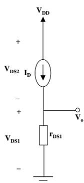
$$I_D = K(V_{GS2} - V_{TH})^2$$
